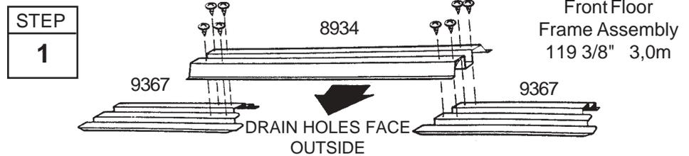
**2** Overlap the **side floor frames** and the **rear floor frames** as shown. The holes in these pieces will align when the pieces are positioned with correct amount of overlap. See the illustrations below for the proper overall length of the side and rear floor frames. Join the frames by inserting four/five bolts into each frame set as shown.
