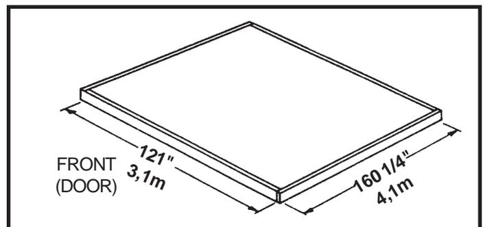
Note: Finished Slab dimensions, with lumber removed.
