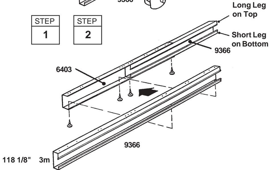
**3** Position **door slides** onto the legs, from the end of door track assembly, as shown in the end view. **NOTE:** Flat side on top, pins and holes **must** be oriented as shown.
