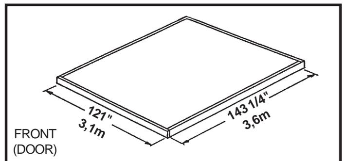
Note: Finished Slab dimensions, with lumber removed.
