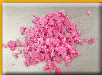
Spilled liquid has been neutralized & absorbed
