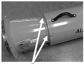
•Remove the 4 sheet metal screws fastening the blower to the duct canister.
