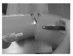
•Once the hose clamp screw is clear of obstruction, continue to slide the duct canister onto the blower.
