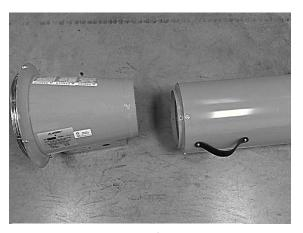
•Separate the blower from the duct canister as shown.
