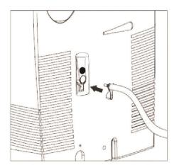
2. Place the other end of the water line (drainage end) into a drain.
