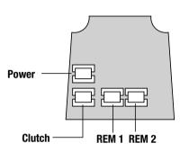
**REM 1** is for connection to a reception desk push button or a door intercom system. Pressing the button will cause the keypad to flash blue on the lock and release the lock for the pre-set time.
