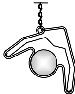
30° Mounting With “Combination” Hanger
