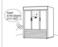
Set the front of the refrigerator a little bit higher than back-side by using adjustable feet to drain the water away with easily.
