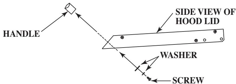
\* Assemble the handle with washers and screws as above drawing.
