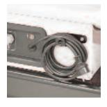
**POWER CORD BRACKET** A bracket on the body is provided for coiling the power cord during transport.
