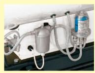
Kit for connecting to external fuel tanks
