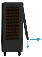
Pull out the bottom of the back panel then take it down.
