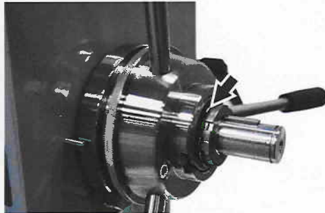
Figure 9 Adjusting the feed switch
