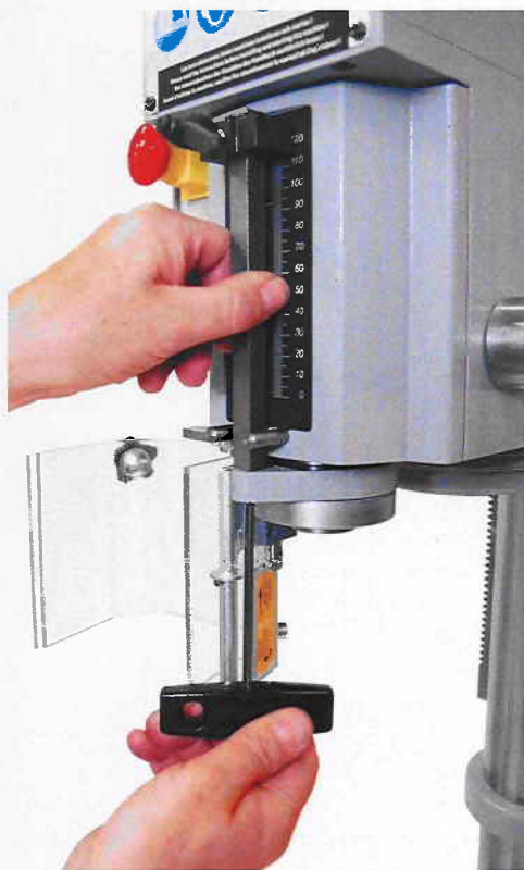
Figure 15 Removing the depth stop rod
