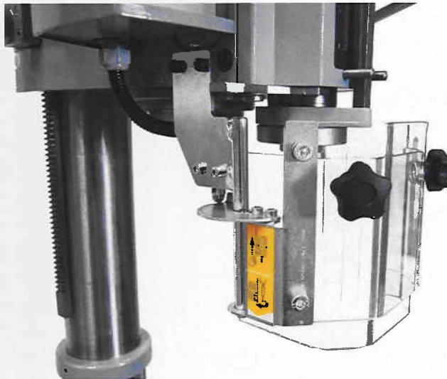
Figure 2 Chuck guard (for machines within the European Union)
