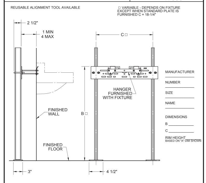
RECOMMEND ALL FEET BE SECURED TO FLOOR WITH 1/2" BOLTS AND ANCHORS BY OTHERS.
