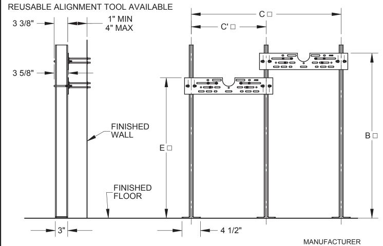
RECOMMEND ALL FEET BE SECURED TO FLOOR WITH 1/2" BOLTS AND ANCHORS BY OTHERS.
