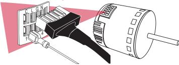
Note the terminal location and corresponding color of each wire that **connects to the blower motor.** A reference diagram is shown below for convenience.
