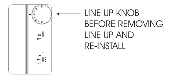
Use special care when removing and re-installing the knob during installation or subsequent servicing.
