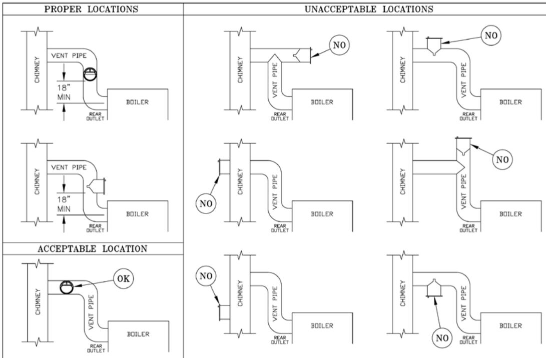
**Figure 16: Proper and Improper Locations of Draft Regulator**
