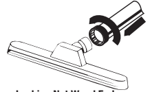
Locking Nut Wand End Insert wand end over nozzle and tighten nut.
