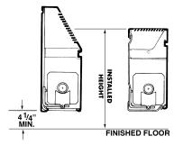
The **installed height** for enclosures is defined as the distance from the finished floor to the center of the outlet. Recommended height is based on a minimum mounting height for all covers and enclosures of 44" from finished floor to bottom of front panel.
