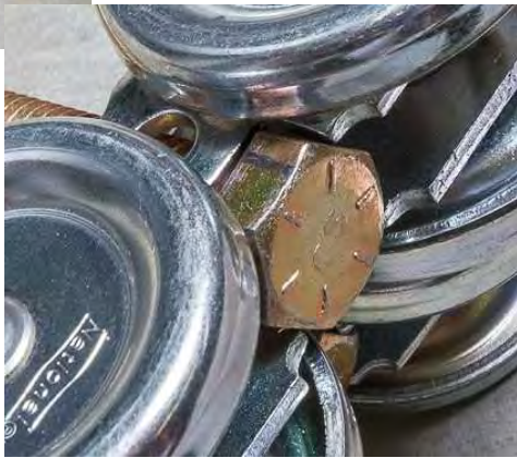
1/2" Bolts shown installed in Roller Assemblies
