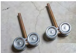
1/2" Bolts shown installed in Roller Assemblies
