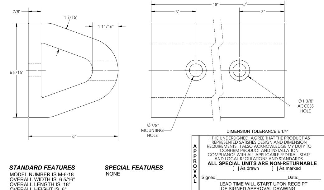
**OVERALL HEIGHT IS 6"** NUMBER OF MOUNTING HOLES 2 MOUNTING HOLE SIZE Ø7/8" ACCESS HOLE SIZE Ø1 3/8" WEIGHT 16 LBS (2)-REINFORCEMENT PLATES INCLUDED SIZE: 1 5/8" x 6"
