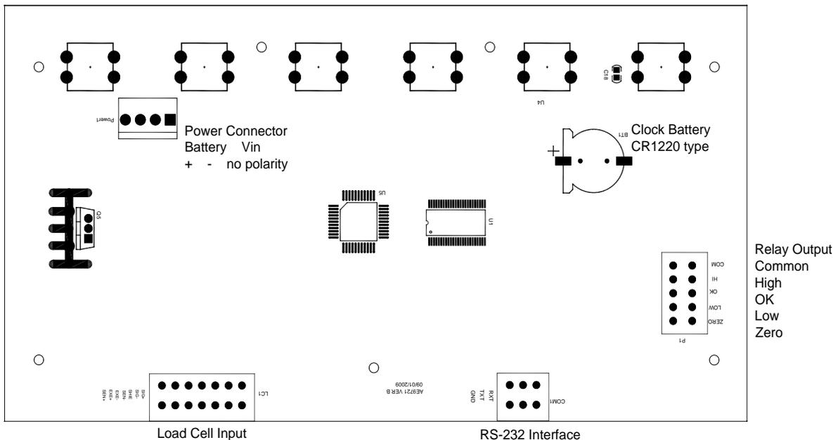
The circuit to control the relays requires an external voltage compatible with the relays used. For more information see section 10.
