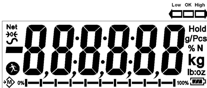
Other symbols will show when a weight has been tared (NET) the scale is at zero and stable, if a value has been stored in memory or when the animal weighing function has been enabled. A battery symbols will show the state of charge of the internal battery.
