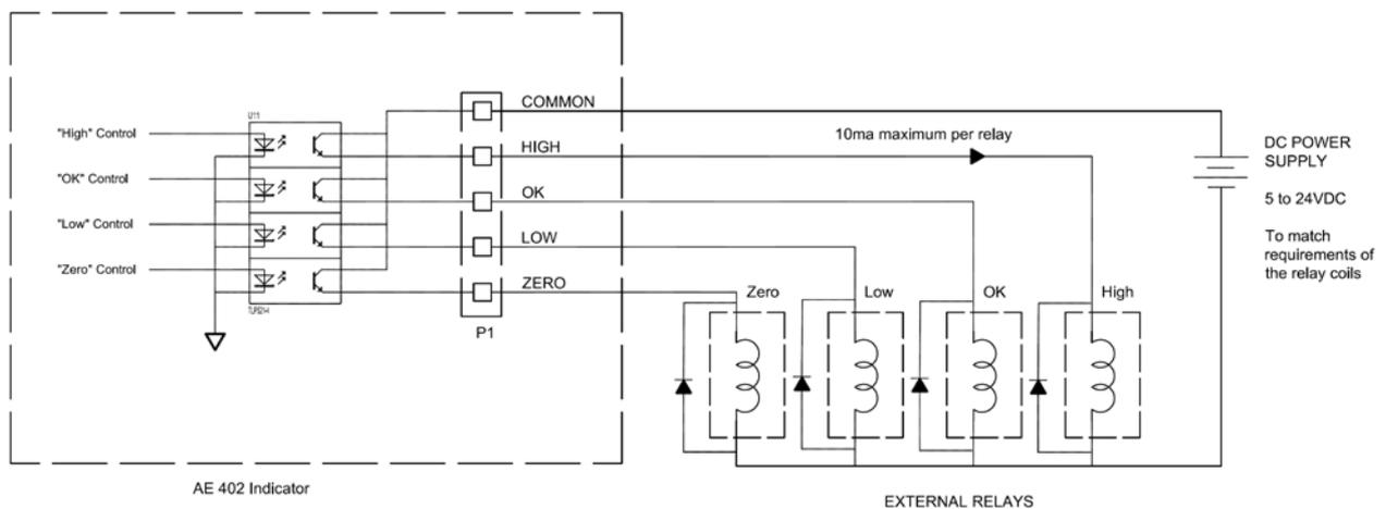
Connections are made to the PCB, Connector P1. The connector is a spring activated type, simply press on the top of the connector and insert the wire.
