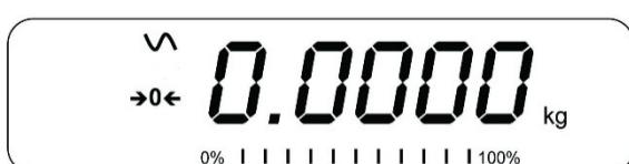
The scales have an automatic re-zeroing function to account for minor drifting or accumulation of material on a connected platform. However you may need to press **[Zero]** to re-zero the scale if small amount of weight is still shown when the platform is empty.
