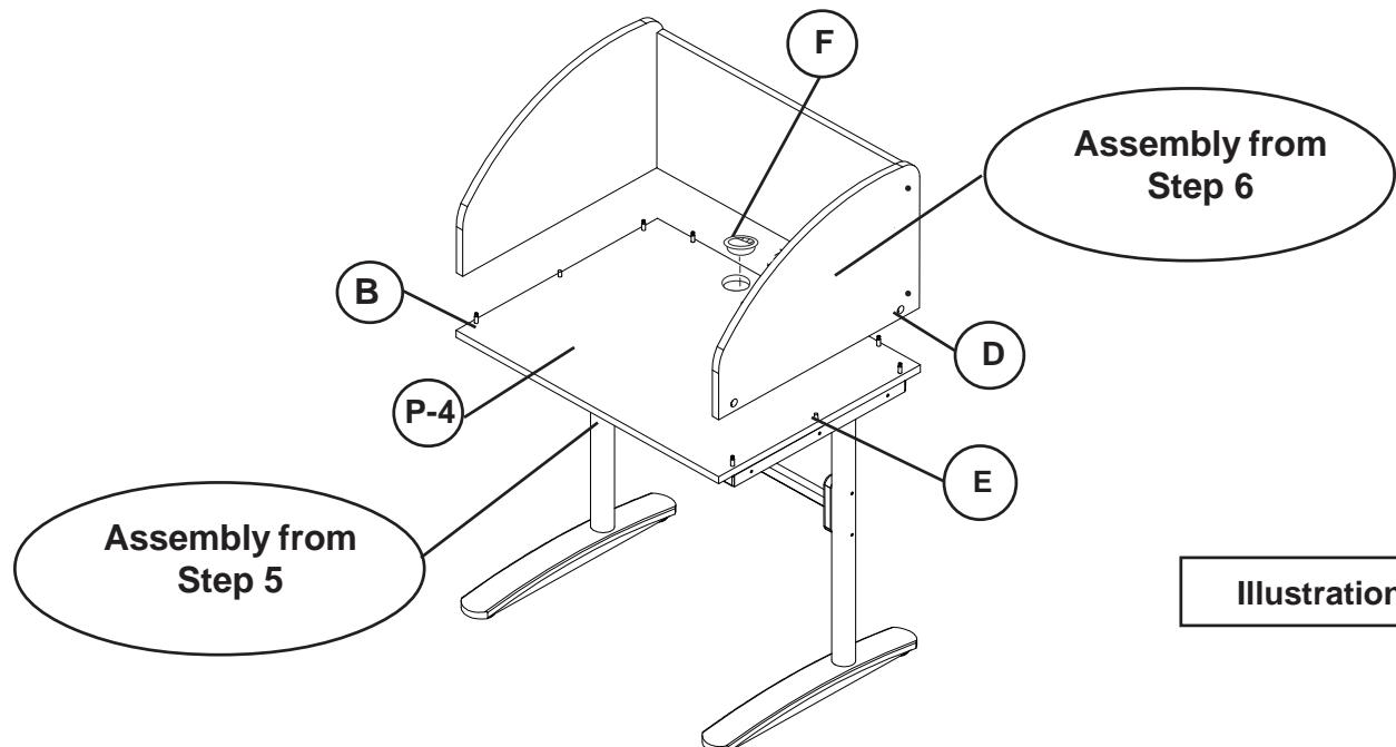
8.) Insert the Top Grommet (F) into the cut-out in the Top Panel (P-4).
