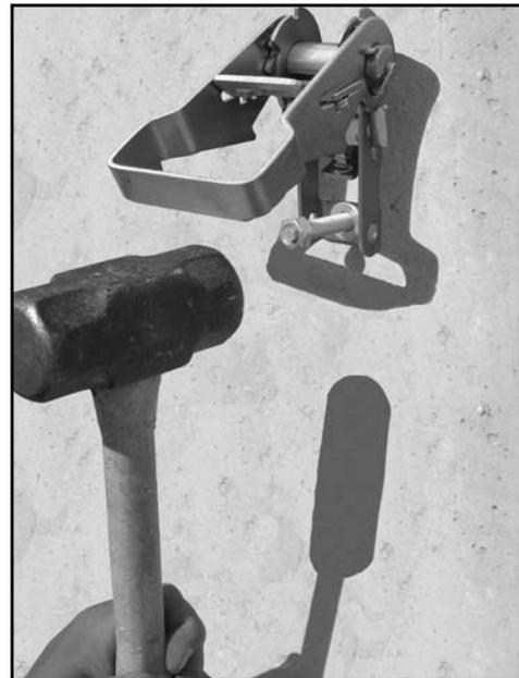
**NOTE:** Depending on wedge anchor bolt, verify that the washer and securing nut are attached *before* driving the anchor bolt into concrete. Striking bolt may cause thread damage and prevent the nut installation.
