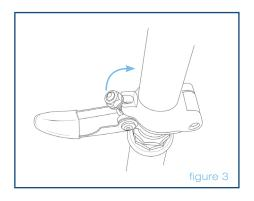
Secure scew and tiller in place by pushing locking handle against the side of the tiller (figure 4).
