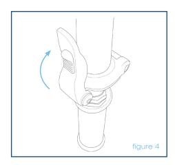
Insert seat post into seat receptacle on frame. Set to desired height and secure in place by inserting thumb screw and turning clockwise until tight.
