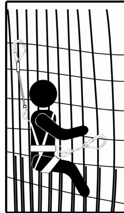
Correct Method for Work Positioning/Tower Work
