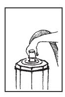
Put backpack on and adjust shoulder straps and waist belt until backpack is comfortable. Harness is made for any custom fit. Attach hose to commercial wand. Attach desired tool to bottom of wand by loosening nut and pushing in tool. Tighten nut until tool is in place. Tool will swivel when using side to side motion. Never take nut off wand or risk loosing metal ring inside the nut. The function of the metal ring is to hold tool in place in its slotted groove.
