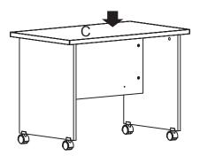
Turn the unit upright. Position the Cams and Dowels of the Worksurface (C) into the Minifix Cams of the unit as shown.
