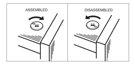
Screw four Minifix Bolts (H1) into the pre-drilled holes of the Worksurface (C) where indicated.
