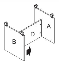
Position the Right Side (B) onto the Back (D) as shown.
