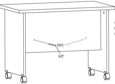
Use an Confirmat Screw (H7) through the Back (D) to secure Paper Rack to unit as shown.
