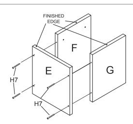
Use four Confirmat Screws (H7) to attach the other Paper Rack Side (E) as shown.
