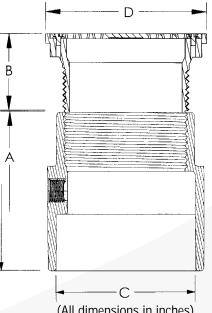
(All dimensions in inches) • Barrel diameter is 3-1/2 in. IPS thread. • Primer tap knock-out is 1/2 in. FIP thread.
