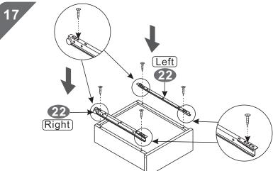
Place the drawer upside-down. Grab the "L" shaped sliders (22) and assemble them to the drawer using Screws (A), with wheels facing towards the back of the drawer. Make sure the sliders are touching the side panels, and that they are not "up in the air".
