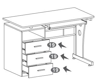
Carefully insert all the drawers starting from the bottom. Make sure the wheels from the drawers engage and roll in the middle of the sliders.
