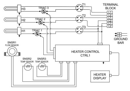
T1, T2, T3 = Thermostat H1, H2, H3 = Heating Element SNSR2 = Inlet Temperature Sensor SNSR3 = Inlet Temperature Sensor
