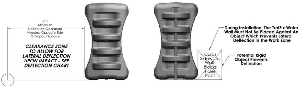
Figure 5: Clear Zone Diagram and Chart Recommendation
