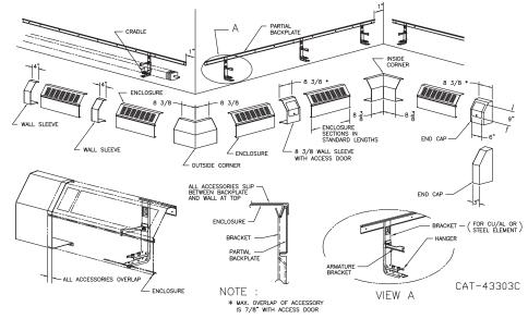
Standard lengths: Available from  $3^{\prime}$  to  $8^{\prime}$  in 12" increments. When two or more covers occur in a run, a  $4^{\prime\prime}$  wall sleeve is to be used at joints.
