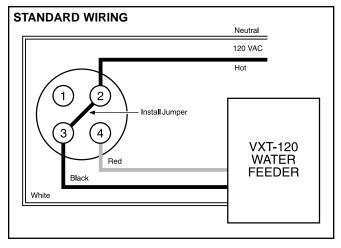
ALTERNATE WIRING: If you choose to wire the feeder to a separate power source from the burner circuit, do not install jumper between 2 and 3. Connect the red wire to 4, the black wire to the hot side of power source and the white wire to common.
