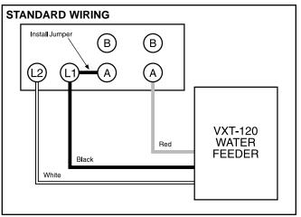
ALTERNATE WIRING: If you choose to wire the feeder to a separate power source from the burner circuit, do not install jumper between L1 and A. Connect the red wire to A, the black wire to the hot side of power source and the white wire to common.
