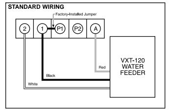
ALTERNATE WIRING: If the power source for the low water cut-off is separate from the burner circuit, remove the jumper between 1 and P1, connect the red wire to A, connect the black wire to the burner circuit hot and the white wire to the burner circuit common.
