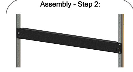
Secure Tool-less Fasteners. If rack screws are used, secure them with screw driver.
