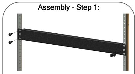
If using cage nut rails, install Tool-less Fastener and / or rack screws on each end of Spacer Blank. If using tapped rails, install with rack screws.
