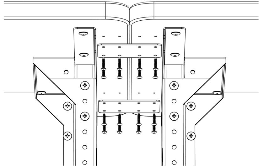
Line up ganging plates with pre-drilled holes on the underside of the front and rear of the training table(s).
