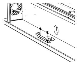
a. Secure the lock base just behind the grommet opening with the 1/4"-20 screws
