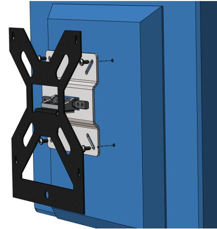
Fasten Monitor to Monitor Mount using Monitor Manufacturer's Screw Specifications.
