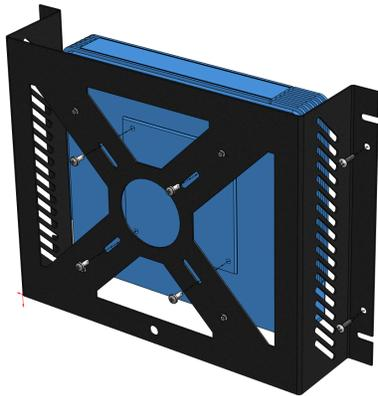
Fasten Thin Client to Back of Wall Mount Base using Screws Provided. Mount Base to Wall using Appropriate Hardware (not included). Fasten to Secure Surface, such as Wall Studs or use Wall Anchors.
