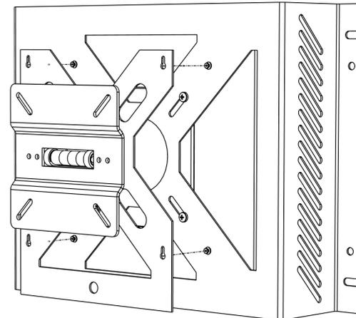
Attach Monitor Mount to Wall Mount Base. Align Keyholes with Fastening Pins. Slide Monitor Mount Down to Secure.
