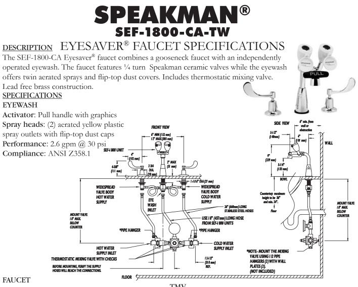
Supply: 1/2" male connections for hot and cold inlets
