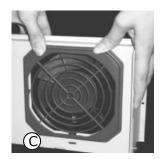
Caution: BFN series products have safety relay switches where the front and rear fan guards attach to the unit. These relays disable the fan/ionizer operation when either fan guard is removed. Take care when attaching the fan guards to assure proper functioning of the product.
