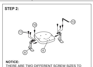
ATTACH THE ARM. USE SCREW (10) FOR INNER HOLES; USE SCREW (11) FOR OUTER HOLES.
