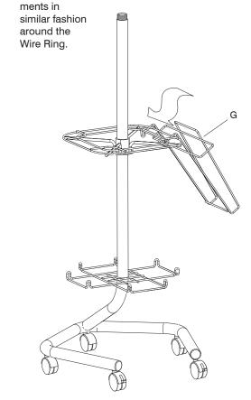
7 Raise the D Lower Wire Ring up so that the hooks of the Lower Wire Ring can be situated over the lower, rear wire of the Wire Compartment as shown below.
