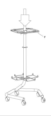
Tilt one of the G Wire Compartments into one side of the Upper Wire Ring. Be sure to engage the upper compartment hook onto the wire ring. Rotate the compartment so it hangs down vertically. Attach three more Wire Compart-
