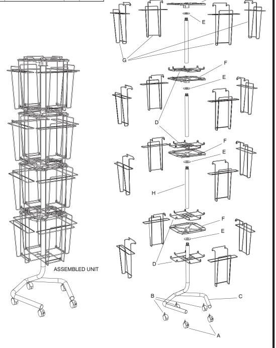
3 Insert two A Casters with Brakes into the bottom of the ends of C Base. Insert three B Casters without Brakes into the remaining holes under the Base.
