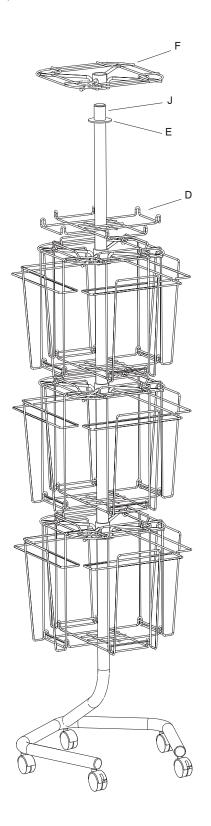
12 Repeat steps 6 – 8 to attach the four remaining Wire Compartments to the Upper and Lower Wire Rings. Your Rotary Literature Display Rack is now ready to use. Simply insert your catalogs, magazines or other forms into the wire compartments. The front casters can be "locked" to prevent the unit from rolling.
