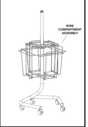
**9** Repeat instructions 4 thru 8 to assemble the second wire compartment assembly.
