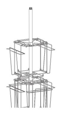
11 For the final wire compartment assembly, slide the remaining D Lower Wire Ring onto the vertical post. Position the E Washer onto the vertical post of the base. Screw the J Short Post with Cap onto the threaded end to sandwich the Washer in position. Place the remaining F Upper Wire Ring over the post to rest on the washer.
