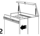
When filing or retrieving, roll the drawer out of the main cabinet to a point where about two inches of the poins remain in the posts of the cabinet.
