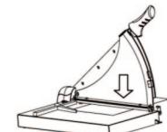
Raise the blade fully to unclamp and (re)move the paper stack.
