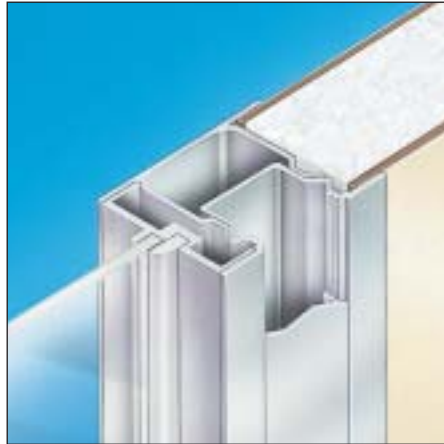
Window-stud-panel detail.
