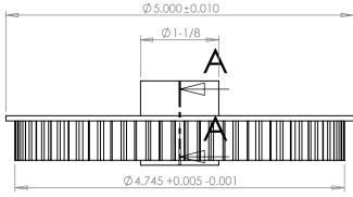
**NOTE: CORED PULLEYS** HAVE 1/16" THICK RIBS, REINFORCEMENT
