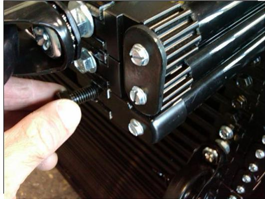
Step #1 Remove 9/16" bolt from bottom of partition
