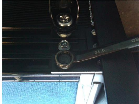
Step #3: Use a 9/16" wrench to tighten bolt.
