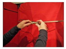
Step #10: Remove the straps holding the partition assembly together.
